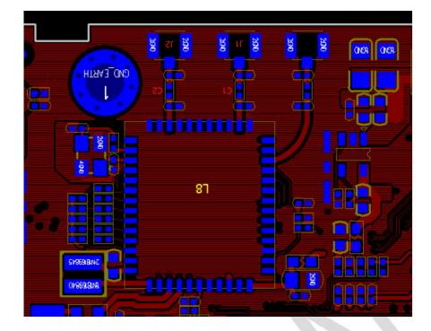
Scrape a GND off the side of the J1&J2,connect the monopole antenna to the PCB at the position of the J1&J2 connector.[The line between the monopole antenna and the WiFi module] must be 50 ohm. C1&C2 is 10pF Capacitors.
