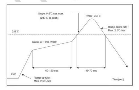
Figure 7. Recommended Reflow for Lead Free Solder
