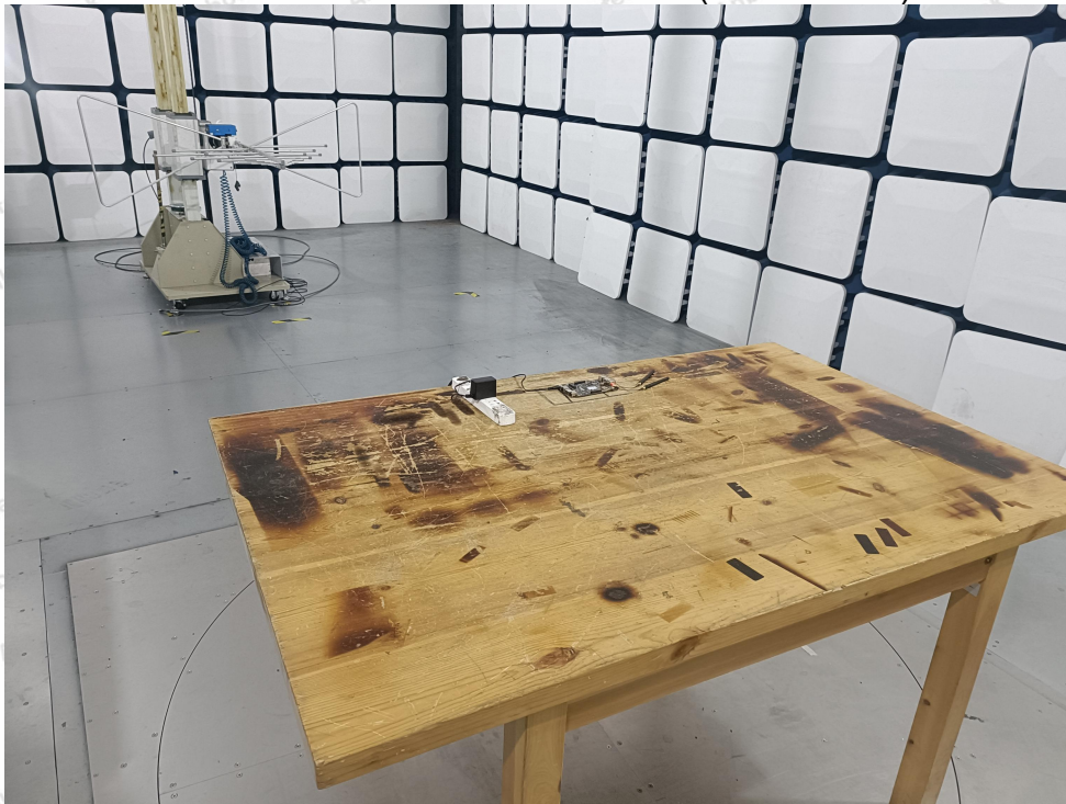
Photo of Radiation Emission Test (below 1GHz)
