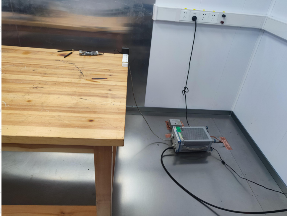
Photo of Radiation Emission Test (below 1GHz)
