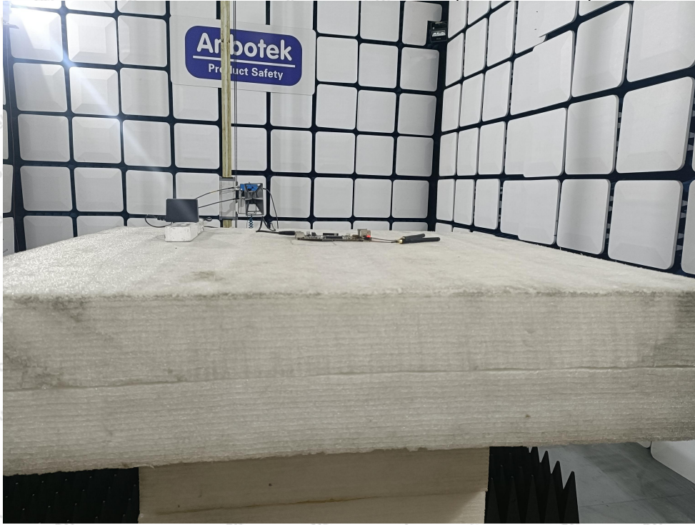
Photo of Radiation Emission Test (above 1GHz)
