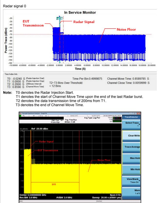
**Note:** An expanded plot for the device vacates the channel in the required 500ms
