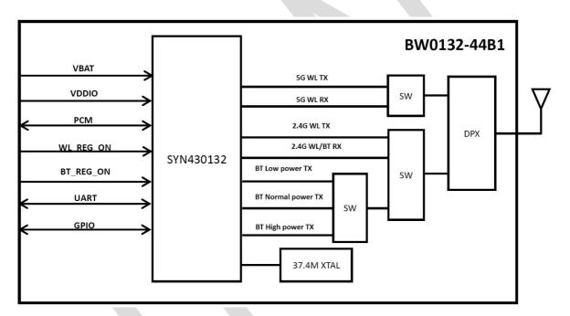
Figure 1. Block Diagram of BW0132-44B1
