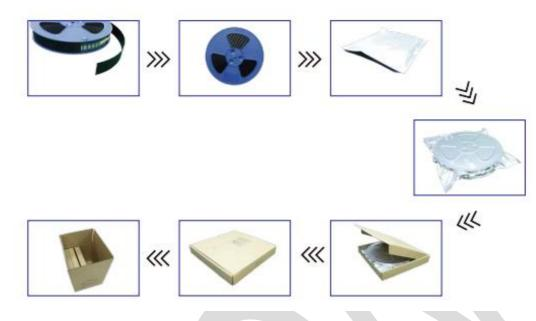
Figure 6. Brief Packaging Process of BW0132-44B1 Modules
