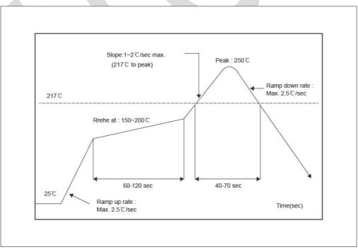
Figure 7. Recommended Reflow for Lead Free Solder
