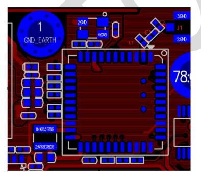
Scrape a GND off the side of the J1, connect the FPC antenna to the PCB at the position of the J1 connector.
