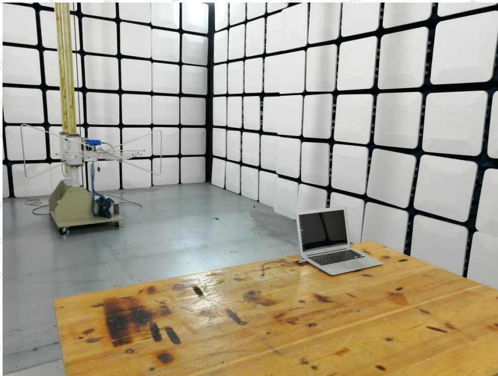
Photo of Radiation Emission Test
