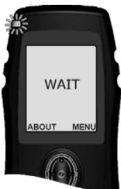
1. The interlock turns on automatically when you plug it in, or when you turn the key to ON. **WAIT** displays as the unit warms up.
