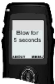
2. The handset displays Blow for 5 seconds when it has finished warming up. The warm-up time may be longer in cold temperatures.
