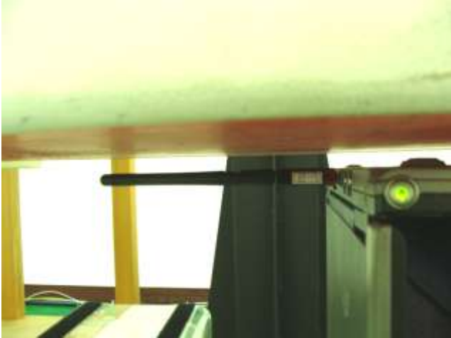
USB Configuration 1 (USB Horizontal-Up with Phantom 1.0 cm Gap and Antenna in Straight mode with 270 degree)
