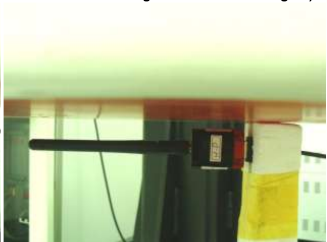
USB Configuration 4 (USB Vertical-Back with Phantom 0.5 cm Gap and Antenna in Straight mode with 270 degree)
