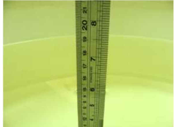
Fig 6.2 Photo of Liquid Height for Body SAR
