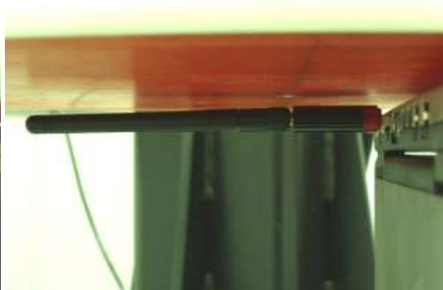
USB Configuration 1 (USB Horizontal-Up with Phantom 0.5 cm Gap and Antenna in Straight mode with 0 degree)
