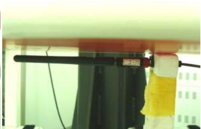
USB Configuration 2 (USB Horizontal-Down with Phantom 0.5 cm Gap and Antenna in Straight mode with 270 degree)
