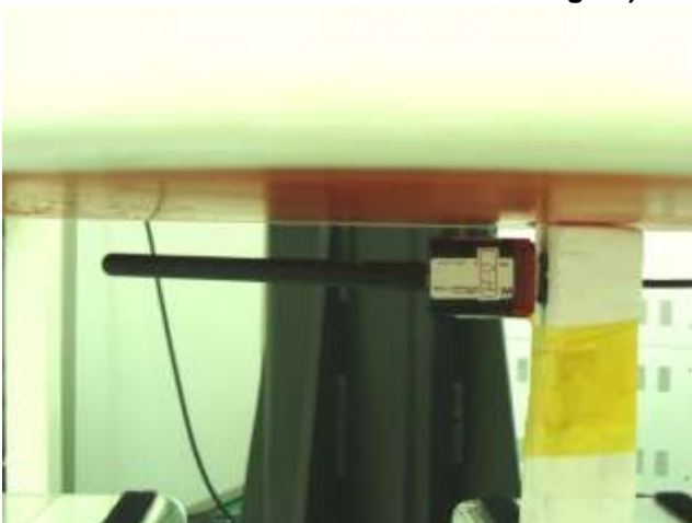
USB Configuration 3 (USB Vertical-Front with Phantom 0.5 cm Gap and Antenna in Straight mode with 270 degree)
