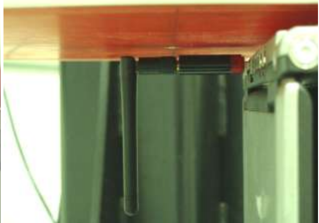
USB Configuration 1 (USB Horizontal-Up with Phantom 0.5 cm Gap and Antenna in Vertical mode with 90 degree)
