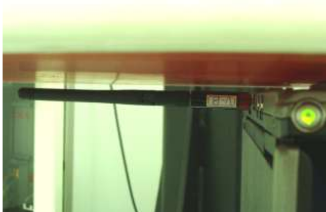
USB Configuration 1 (USB Horizontal-Up with Phantom 0.5 cm Gap and Antenna in Straight mode with 180 degree)
