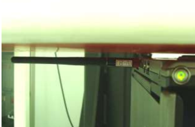
USB Configuration 1 (USB Horizontal-Up with Phantom 0.5 cm Gap and Antenna in Straight mode with 0 degree)
