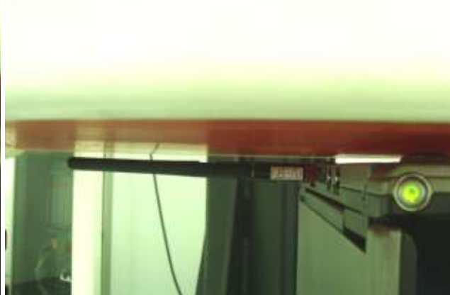
USB Configuration 1 (USB Horizontal-Up with Phantom 0.5 cm Gap and Antenna in Straight mode with 180 degree)
