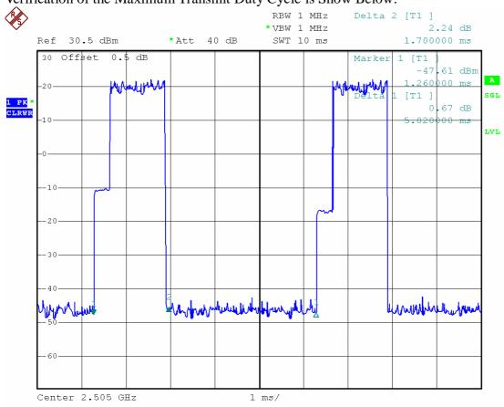
Time for one complete transmit cycle is 5.02msec.
