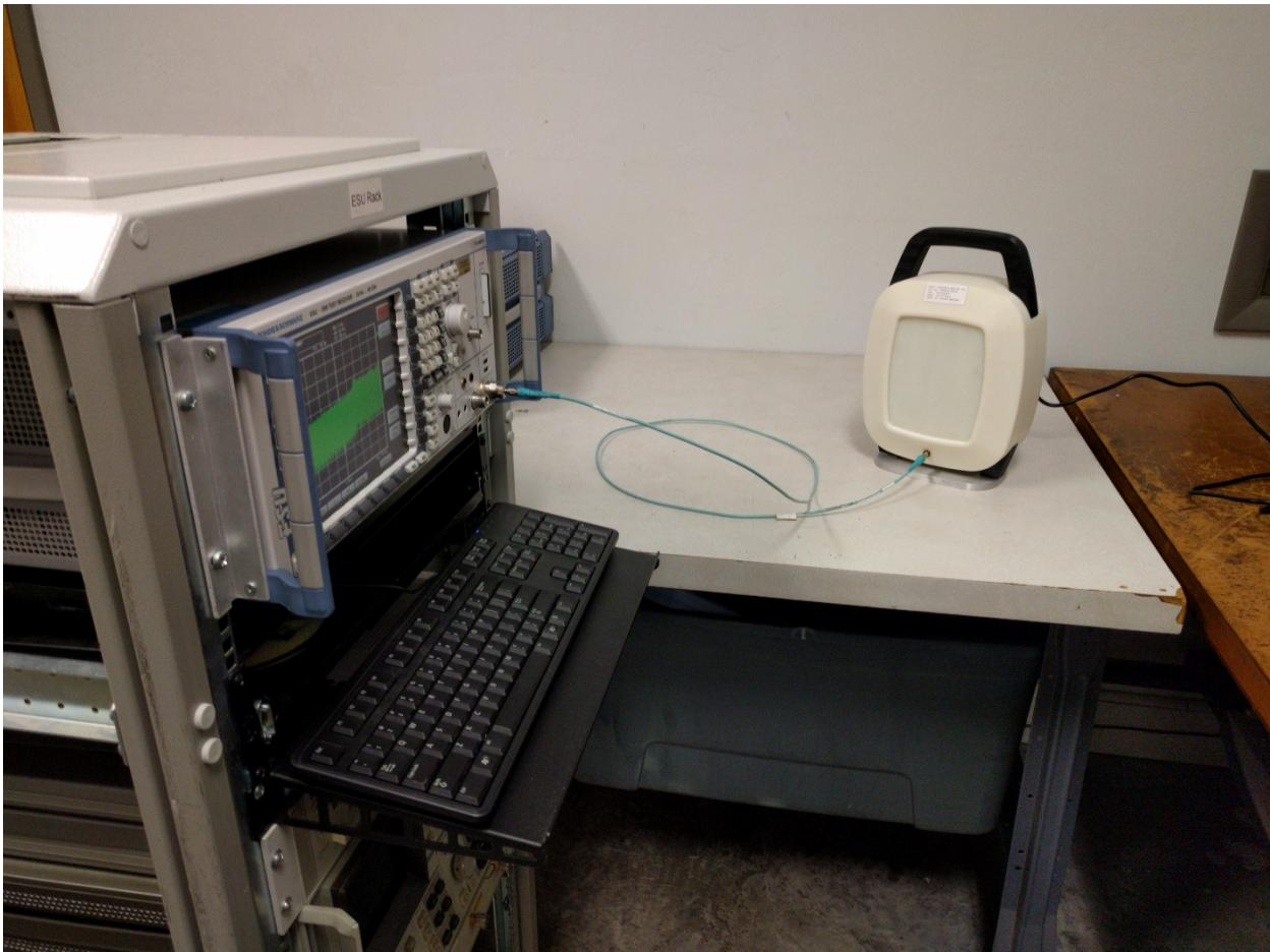
**FIELD STRENGTH OF SPURIOUS EMISSIONS – FINAL SETUP**
