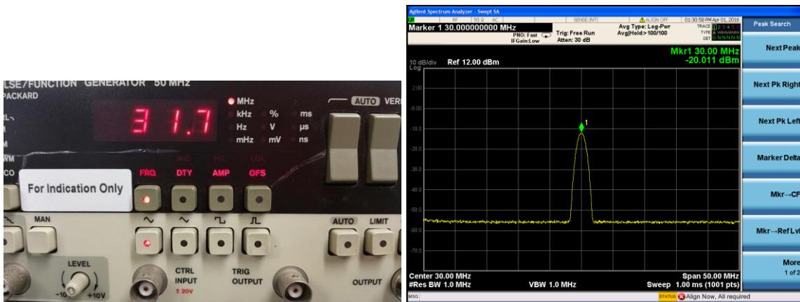
Set the function generator to sine wave, change the frequency till the peak of the output is at 30MHz. As you can see in the picture the function generator is set to 31.7MHz to get the 30MHz output, the numbers and output don't quite tie up which is why the calibrated spectrum analyzer is used to check / setup the output. Once the frequency is set adjust the AMP setting to adjust the output power to -20dBm.
