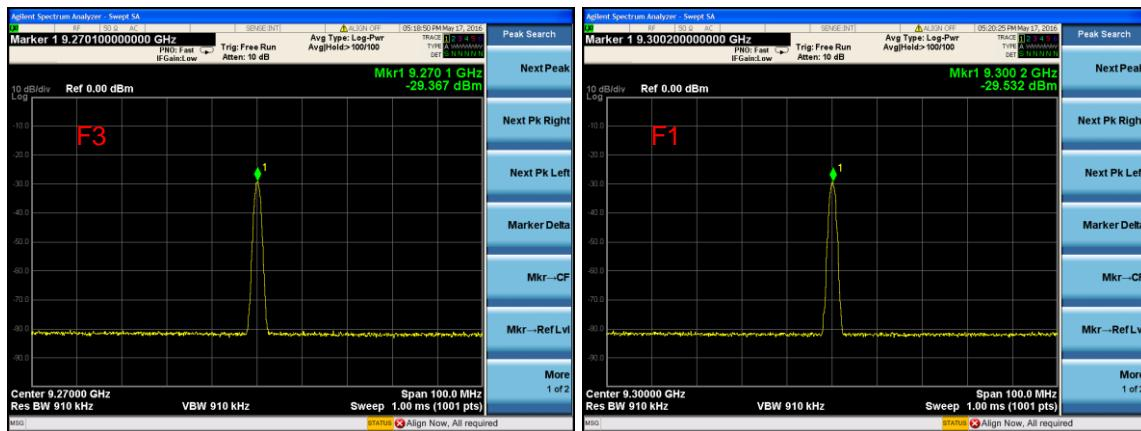
Select the remote stations in the ASI for F2, F3 and F1 and move the centre frequency on the spectrum analyser to suit. You will see the above output power peaks at each frequency setting, use peak search on the spectrum analyser to measure each frequency.
