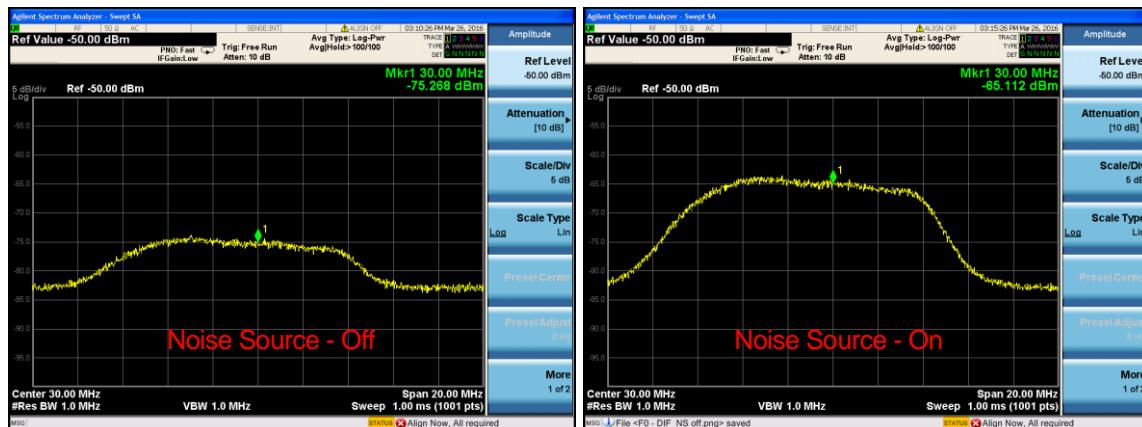
With the noise source powered off, you will get a flat filter response shown above. If the filter response is not flat then there is something wrong in the build.
