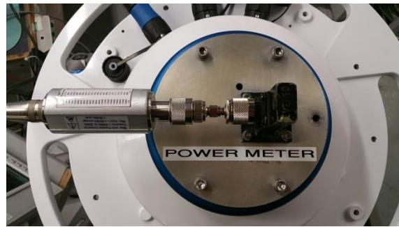
Place in Standby, remove 30dB attenuator and connect the power meter directly to the power meter adaptor plate. Set dB REL to -16.8dB on the power meter, this is the loss of the waveguide adaptor only.
