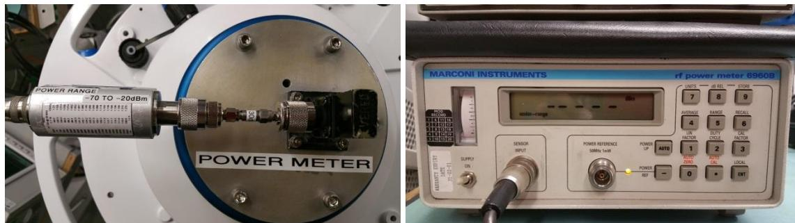
Set the power meter up (If using TE500, power head 6920):
