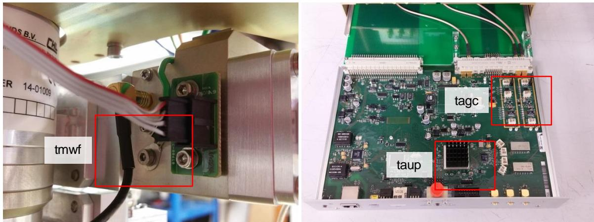
The taup and the tagc temperature sensors are on board the AUP. Remove the AUP and slot in the AUP breakout board. To test these you don't need to remove the top cover of the AUP enclosure (Picture shows areas to spray) and spray each of the sensor areas with freezer spray for a fraction of a second (prolonged spraying can cause thermal damage) watch the temperature on the ASI drop and recover by a few degrees.
