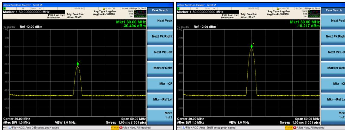
Each time you change the attenuator check on the spectrum analyzer that the signal is correct. As you change the attenuators the signal strength will follow suit, the frequency will always be at 30MHz. When all attenuator values have been done, return to the original -20dB attenuator.
