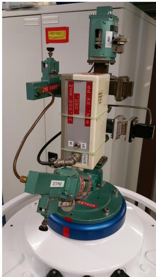
Turn 'On' the horses head and it should start to rotate. Using the delta phase and 180 phase adjustments you can get the horses head to rotate both clockwise and anticlockwise. This will take a bit of playing with to find the best adjustment place for maximum output.
