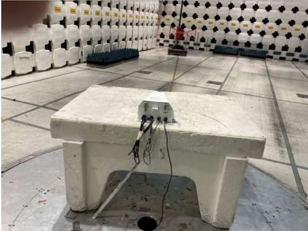
Radiated Test Setup, 30-1000 MHz
