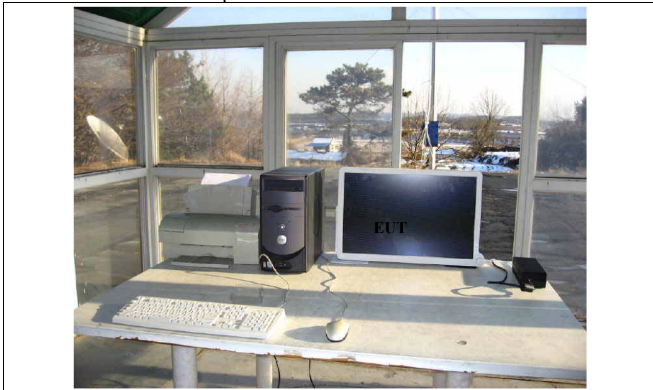
Figure 5 Photo of Radiated emission test setup: DVI Mode
