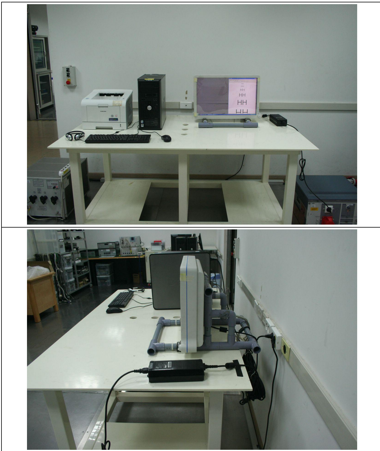
Figure 1. Conducted Emission Test Setup for DVI Mode:
