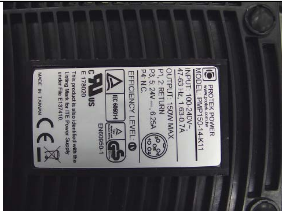
AC/DC Adapter Label (Manufacturer: Protek Model: PMP150-14-K11)
