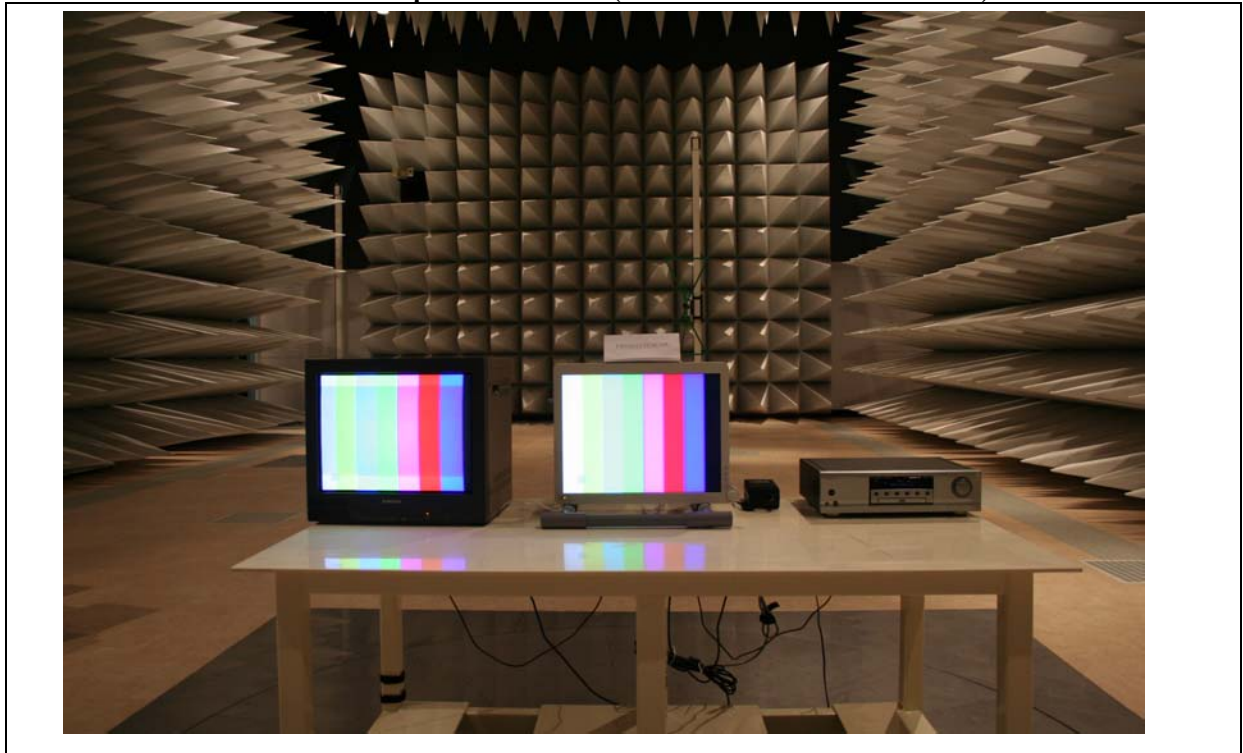
Figure 10 Photo of Radiated emission test setup: S-Video Mode (LCD Panel: TX54D31VC0CAB)
