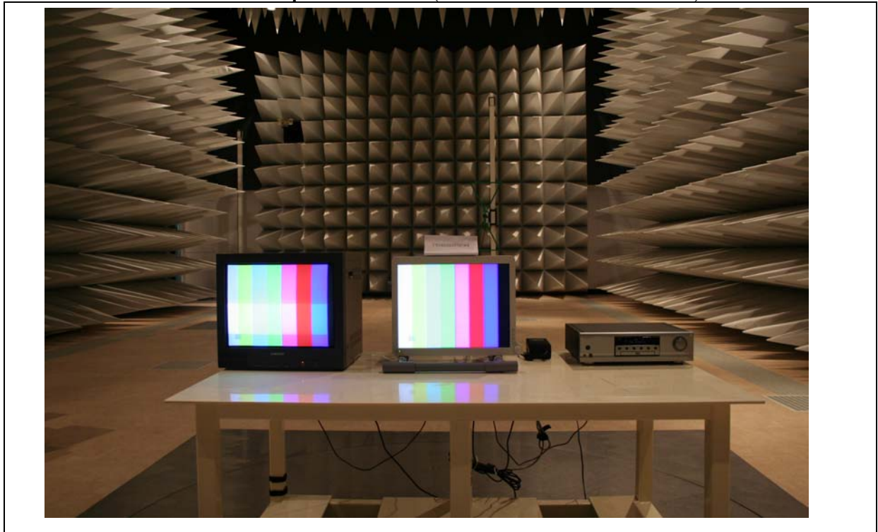
Figure 12 Photo of Radiated emission test setup: S-Video Mode (LCD Panel: TX54D32VC0CAA)
