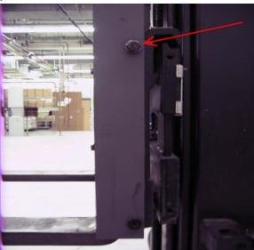
2. Insert the Primary Assembly from the rear of the LBR and secure down using four 5/16-18 1" black oxide button-head bolts.
