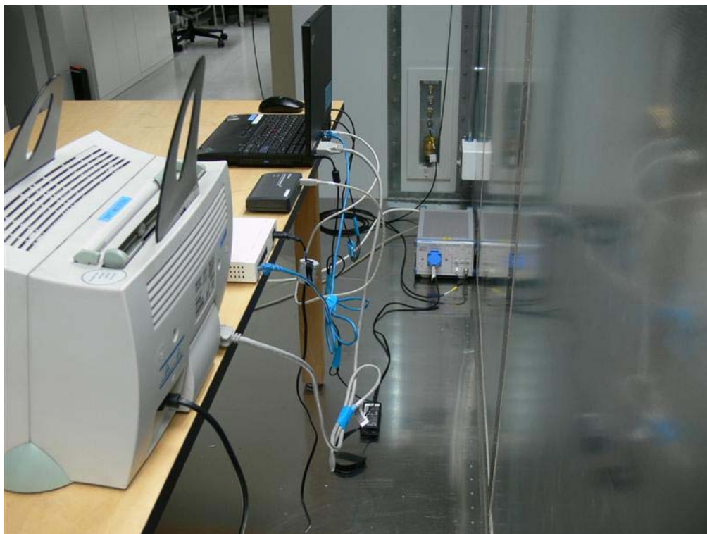
Photograph 5: Set-up for AC Mains Conducted Emission, Rear View
