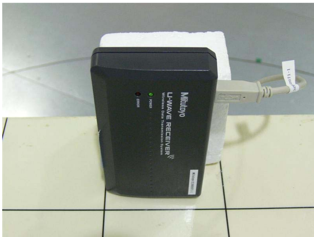
Photograph 3: Set-up for Radiated Emission, EUT Configuration Z-Axis
