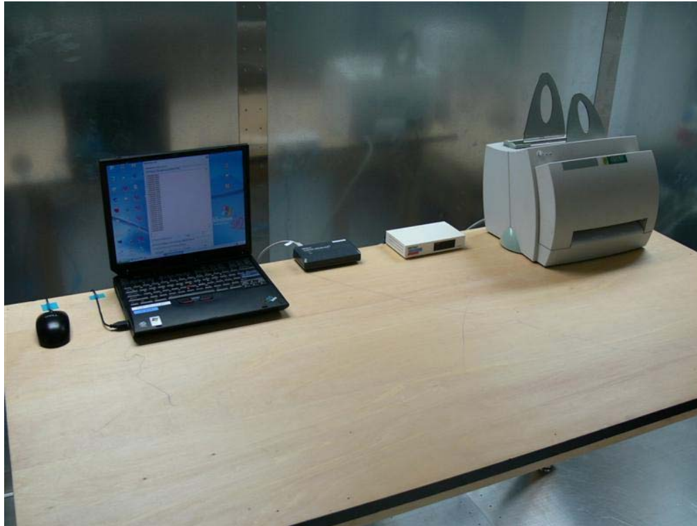
Photograph 4: Set-up for AC Mains Conducted Emission, Front View
