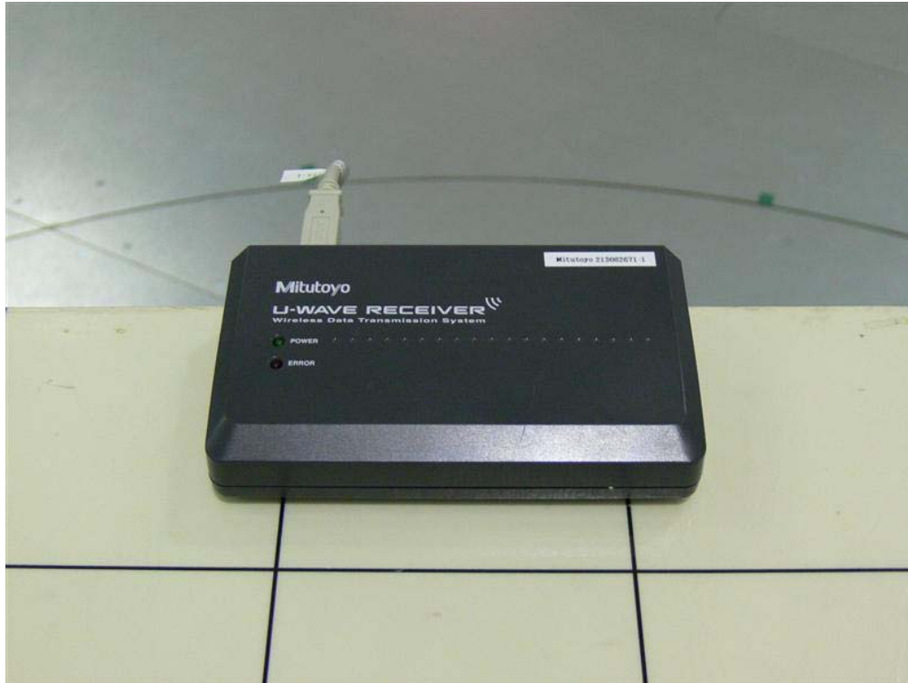
Photograph 1: Set-up for Radiated Emission, EUT Configuration X-Axis
