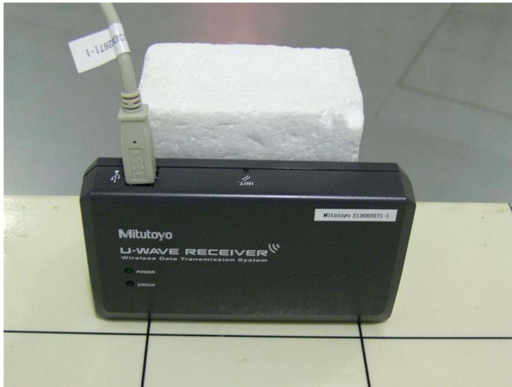
Photograph 2: Set-up for Radiated Emission, EUT Configuration Y-Axis
