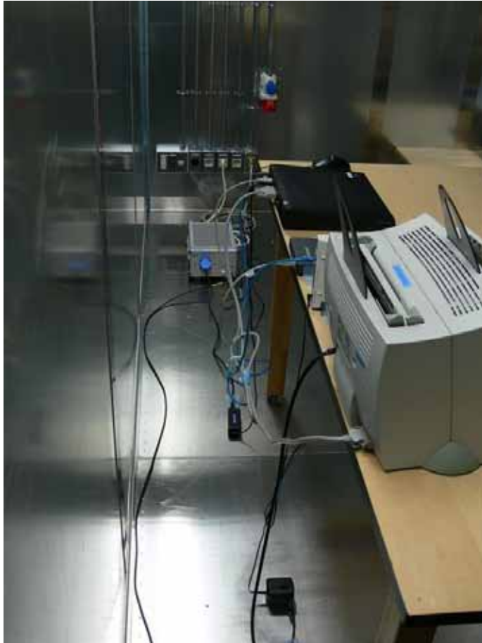
Photograph 1: Set-up for Conducted Emission, on AC Mains (Rear)
