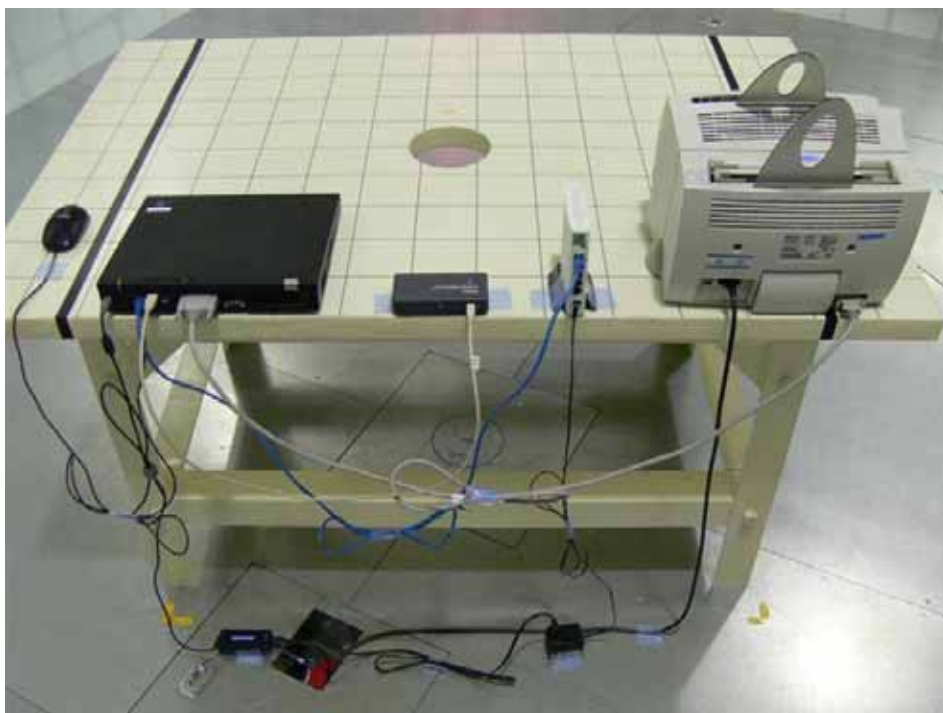
Photograph 3: Set-up for Radiated Emission (Rear)
