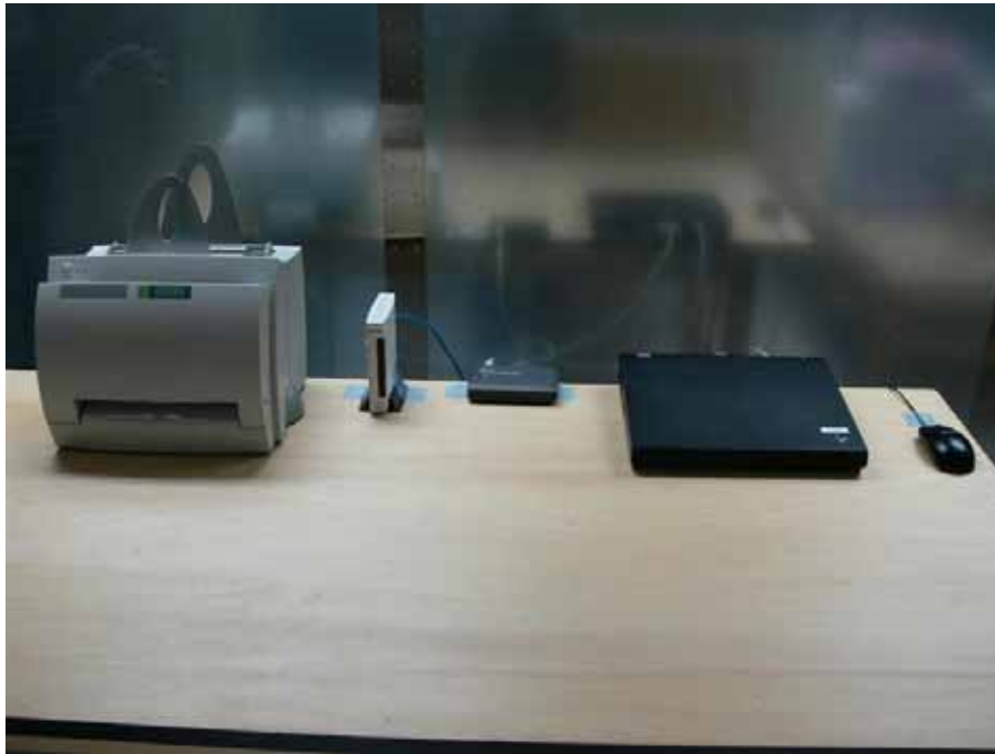
Photograph 2: Set-up for Conducted Emission, on AC Mains (Front)
