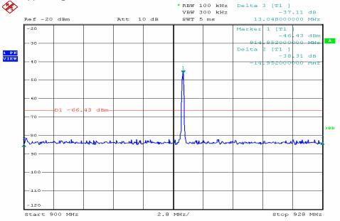
TEST RESULTS: The unit does meet the FCC requirements.
