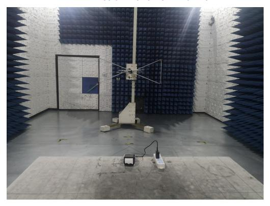
RADIATED EMISSION TEST SETUP ABOVE 1GHz
