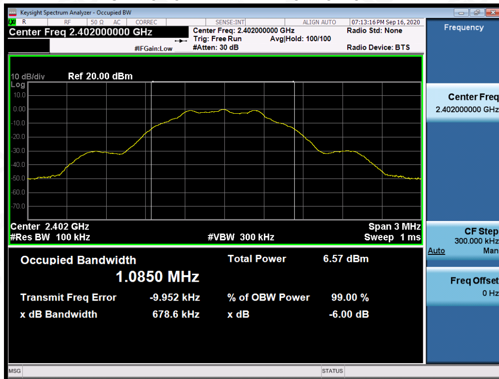
TEST PLOT OF BANDWIDTH FOR LOW CHANNEL
