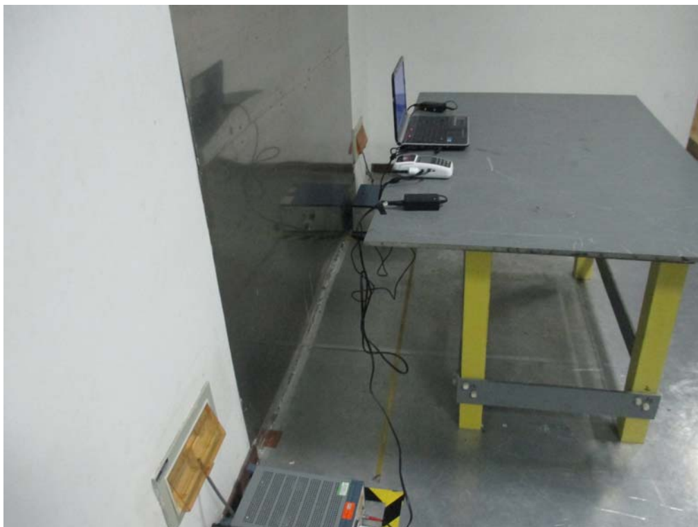
Conducted Emissions Test Setup Side View
