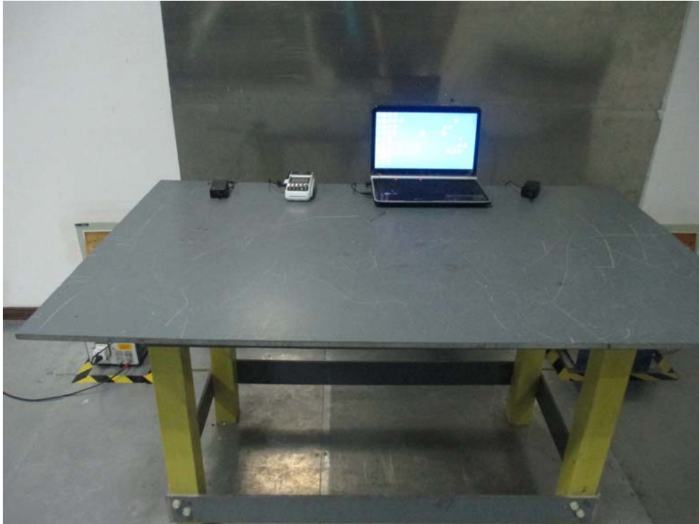
Conducted Emissions Test Setup Front View
