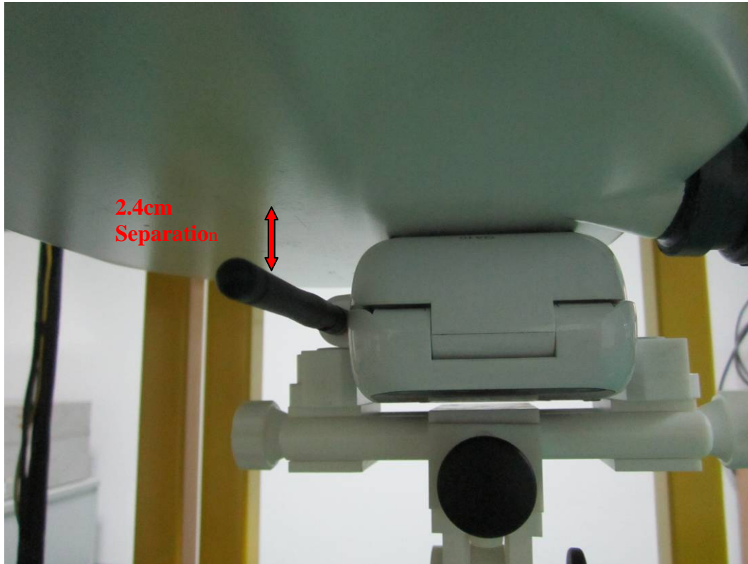
Body Setup Photo (Antenna 90 degree)
