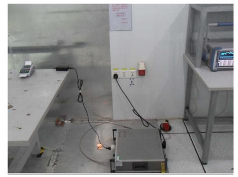
4.1. Photo of Power Line Conducted Emission Test
