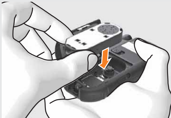
15 Re-insert the test cassette into the meter.
