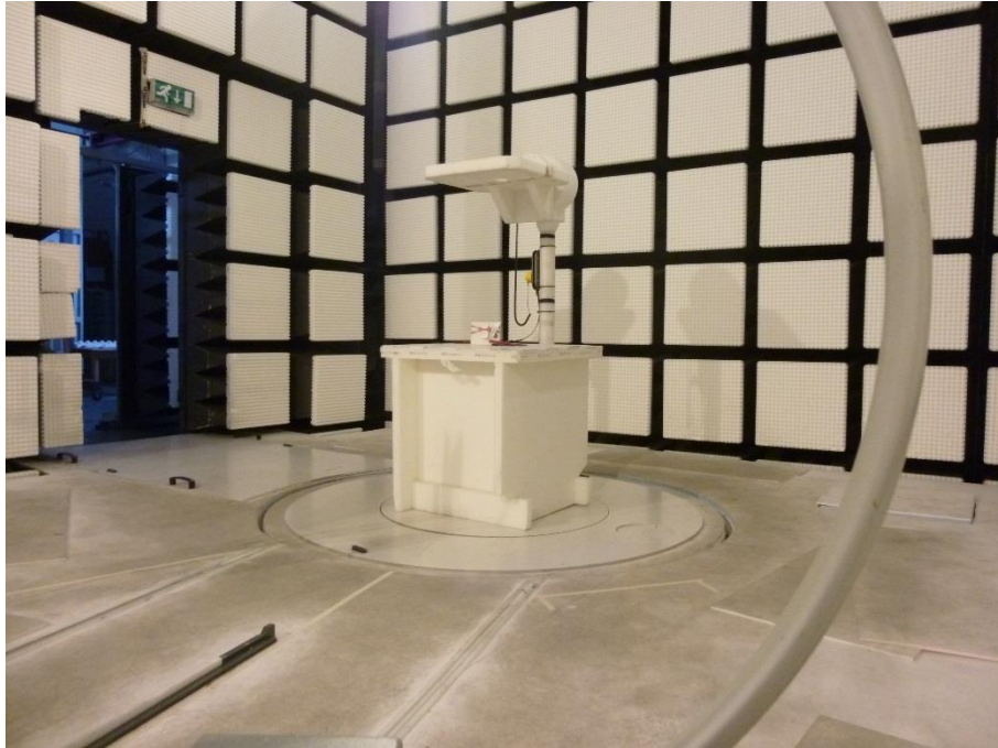
Photo 9: EUT at the anechoic chamber, loop antenna test setup
