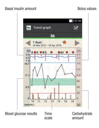
On the **upper left side** (U) of the graph, the basal amount is displayed. By means of the scale, you can read the basal insulin amounts, which are represented by the blue basal insulin line. Scaling depends on the largest basal insulin amount delivered during the selected time period.
