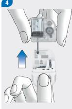
Remove the used reservoir from the pump base.
