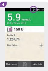
The  $\rightarrow$  symbol in the status bar indicates that flight mode is turned on.
