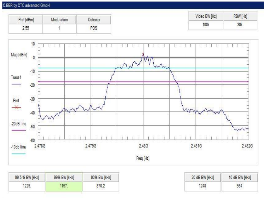
Plot 6: highest channel – 2480 MHz, Pi / DQPSK modulation
