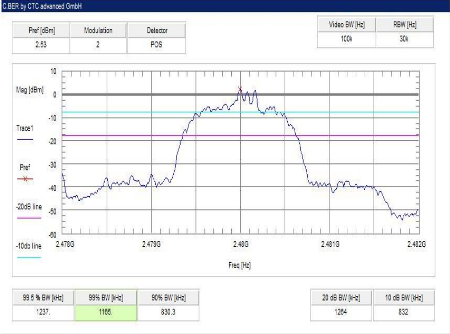
Plot 9: highest channel – 2480 MHz, 8 DPSK modulation
