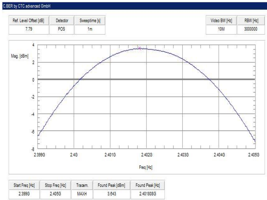
Plot 4: lowest channel – 2402 MHz, Pi / DQPSK modulation
