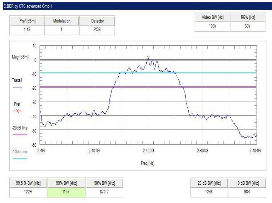
Plot 4: lowest channel – 2402 MHz, Pi / DQPSK modulation
