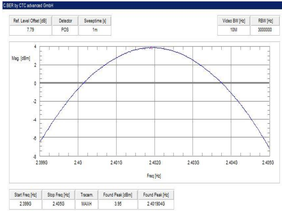
Plot 7: lowest channel – 2402 MHz, 8 DPSK modulation
