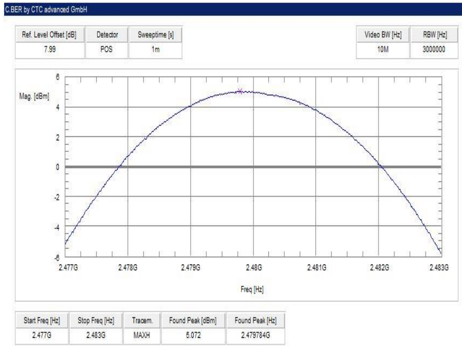
Plot 6: highest channel – 2480 MHz, Pi / DQPSK modulation
