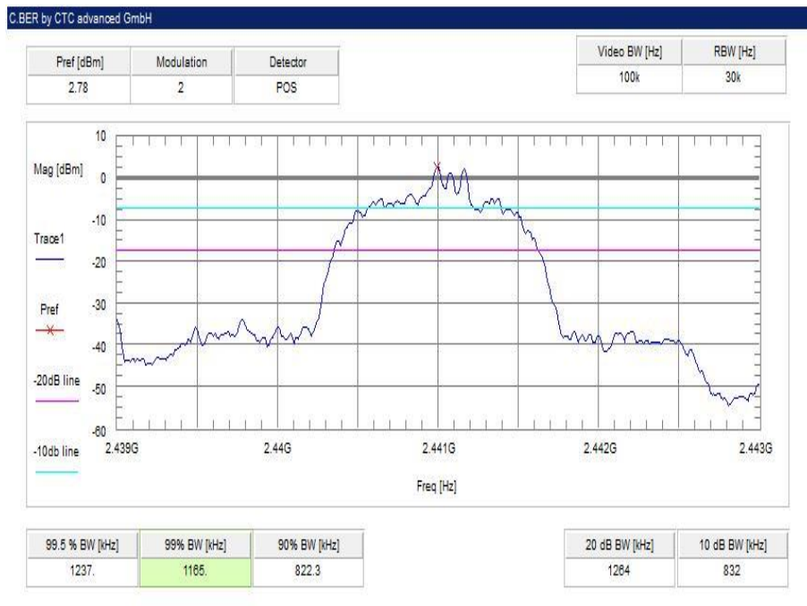
Plot 8: middle channel – 2441 MHz, 8 DPSK modulation
