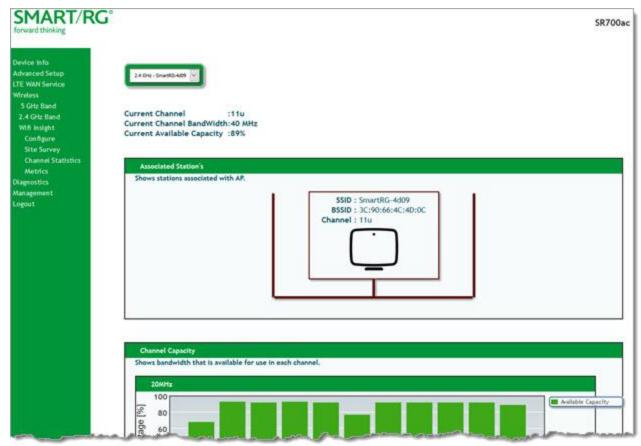
2. In the field at the top of the page, select the wireless band to review. Information is shown for associated stations, channel capacity, interference levels, adjacent channels, and channel distribution.
