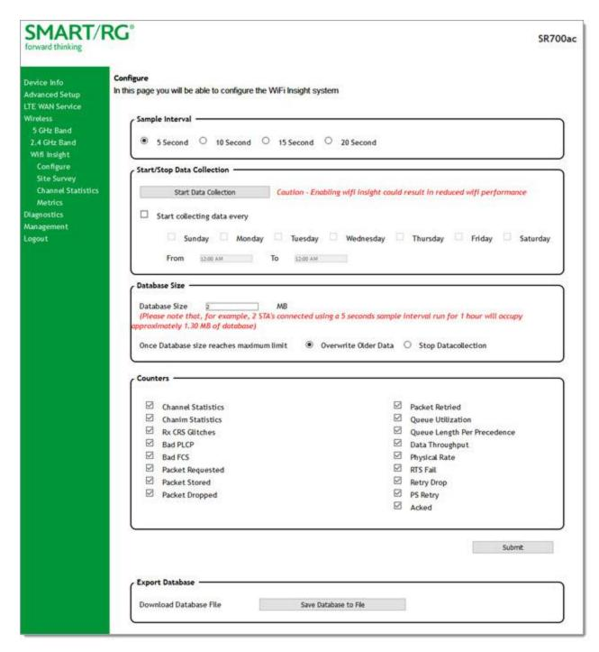
2. In the Sample Interval section, select the number of seconds for sampling to occur. Options are 5, 10, 15, and 20 seconds. The default is 5 seconds.
