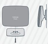
Slide the mount onto the back of the gateway. Tighten the screw located in the bottom of the mount.
