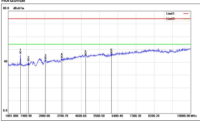
Test Mode: TX / IEEE 802.11n HT20 MHz (CH Mid)
