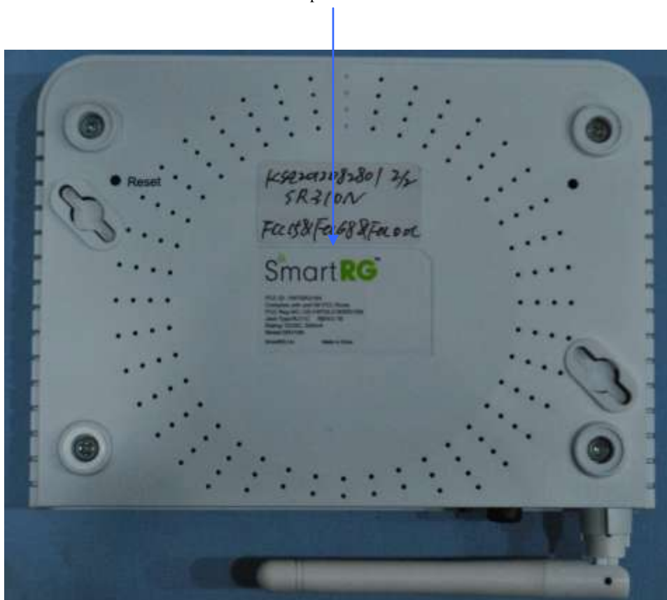
EUT Bottom View/Proposed FCC ID Label Location
