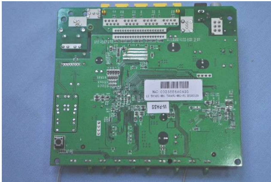
Main & RF board solder side
