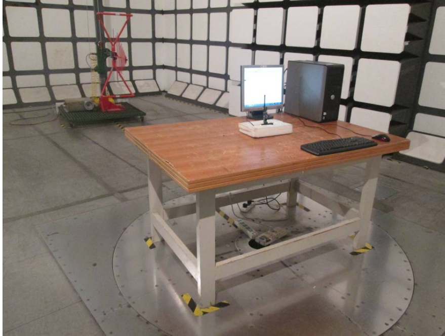
Radiated Emissions View (Below 1 GHz)
