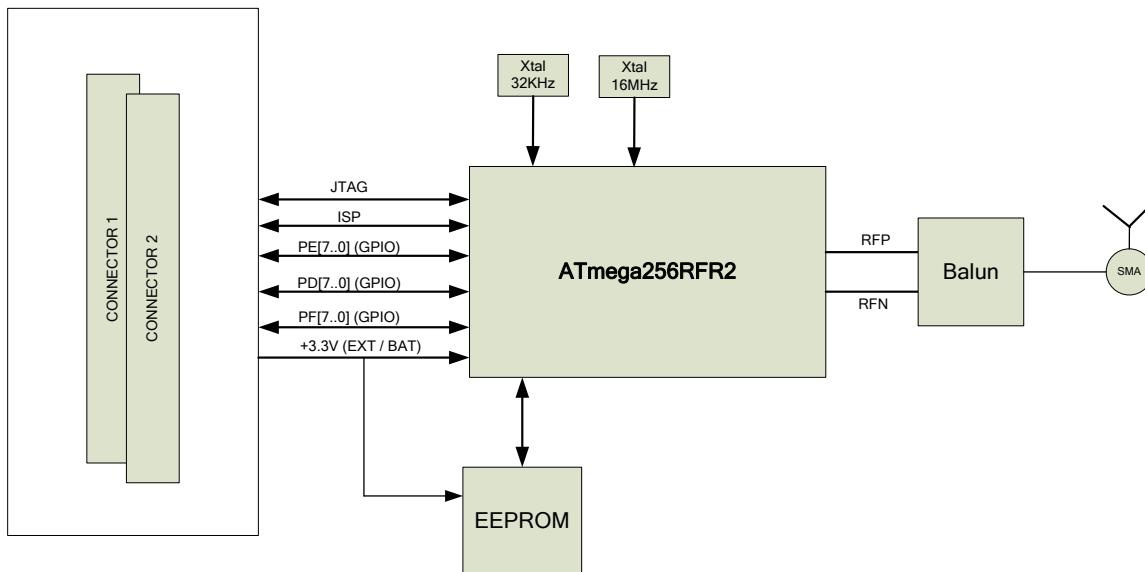
Internal Block diagram of **ATmega256RFR2** RF Transceiver IC, showing Internal Voltage Regulator – AVREG, DVREG
