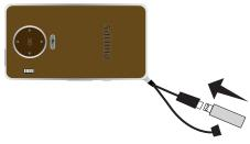
Connect the USB storage medium to the USB cable of the device.
