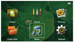
**Source** – Switch to the external video input **HDMI** or select WiFi (if WiFi dongle connected)
