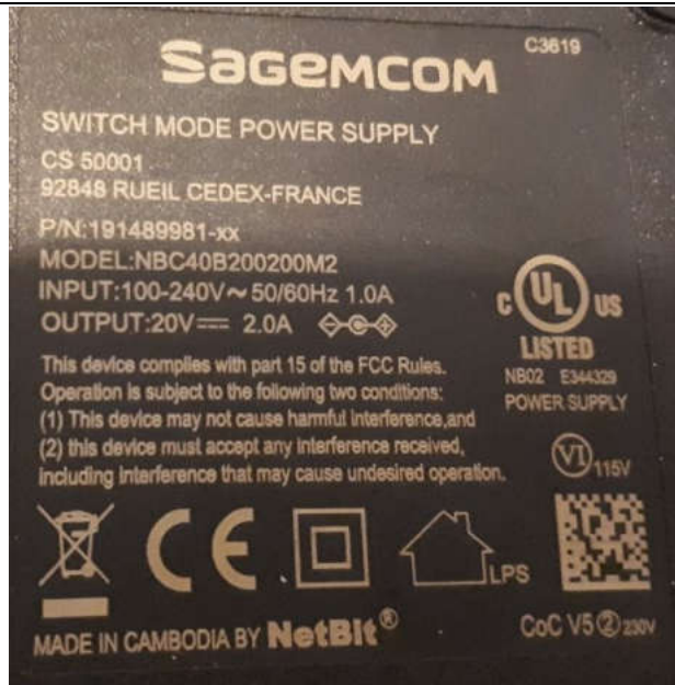
Power supply Marking Plate
