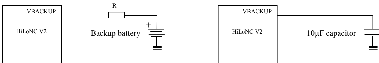
Figure 28: Backup battery or 10µF Capacitor internally charged
