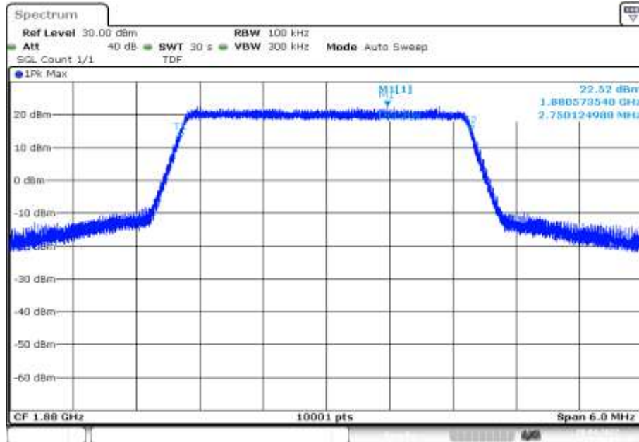
Plot 81: 3 MHz – 64-QAM - middle channel (99% - OBW)
