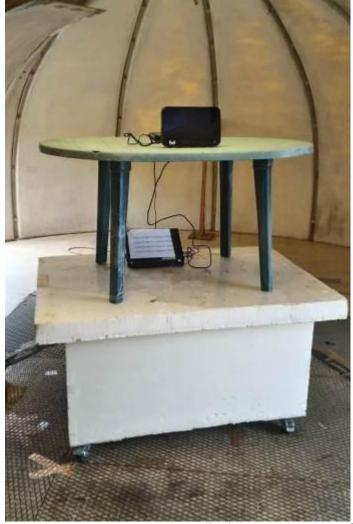
Test setup for radiated emissions test (for frequencies above 1GHz)
