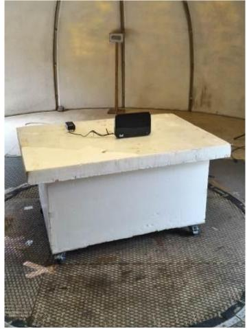
Test setup for radiated emissions test (for frequencies below 1GHz)
