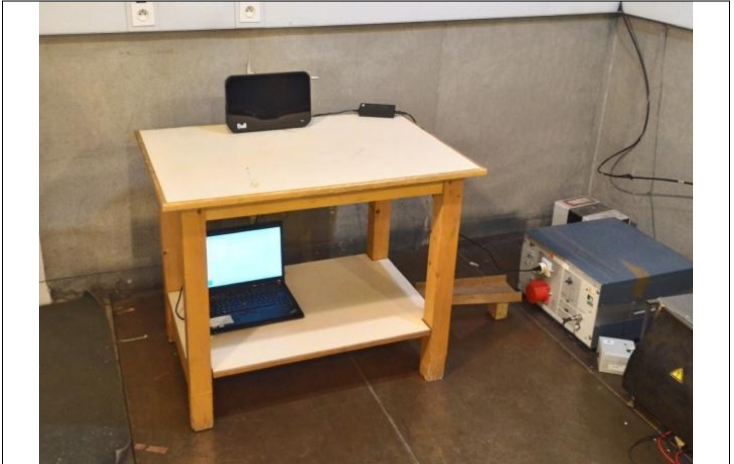
Photograph for AC Power Line Conducted Emissions (Front view)
