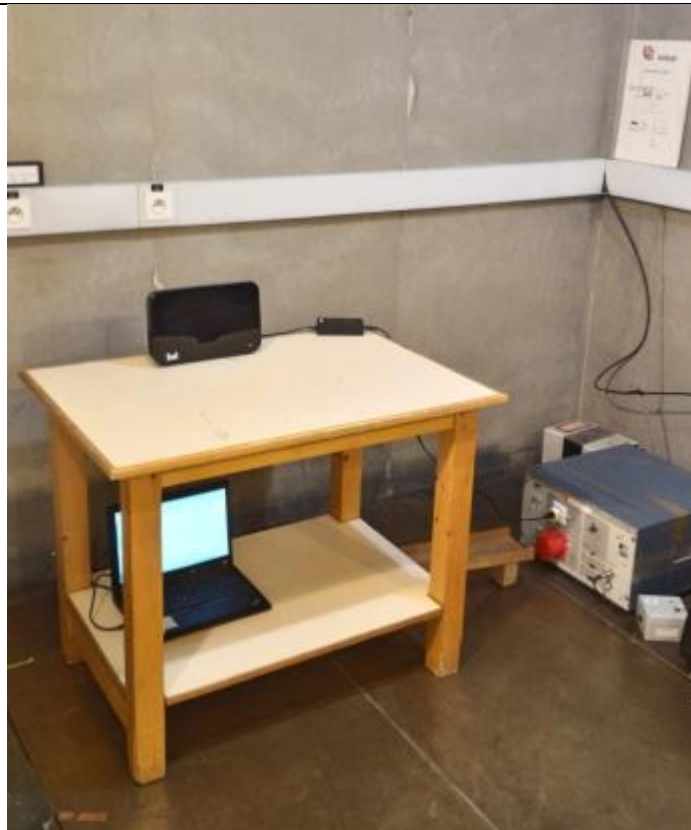
Photograph for AC Power Line Conducted Emissions (Front view)
