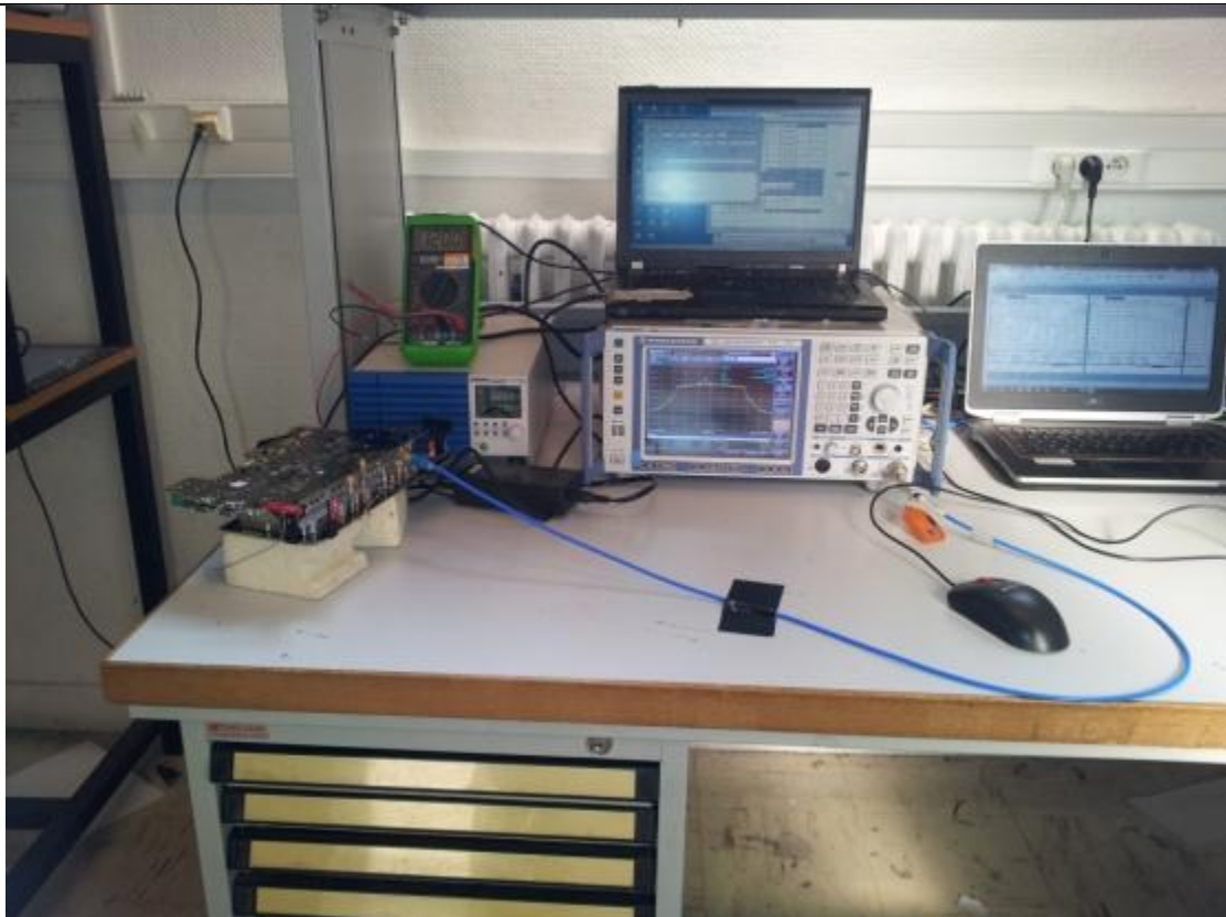
Photograph for 6dB emission bandwidth
