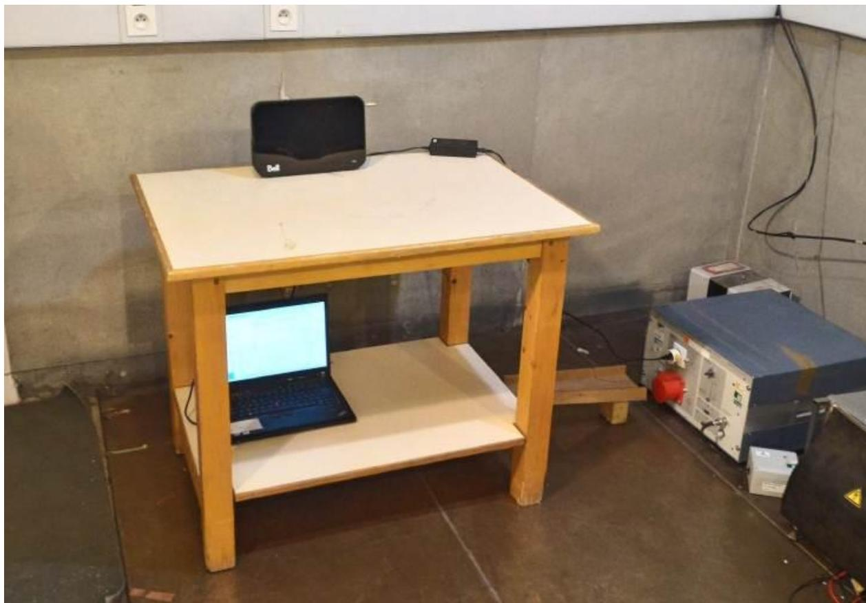
Test setup for conducted emissions test
