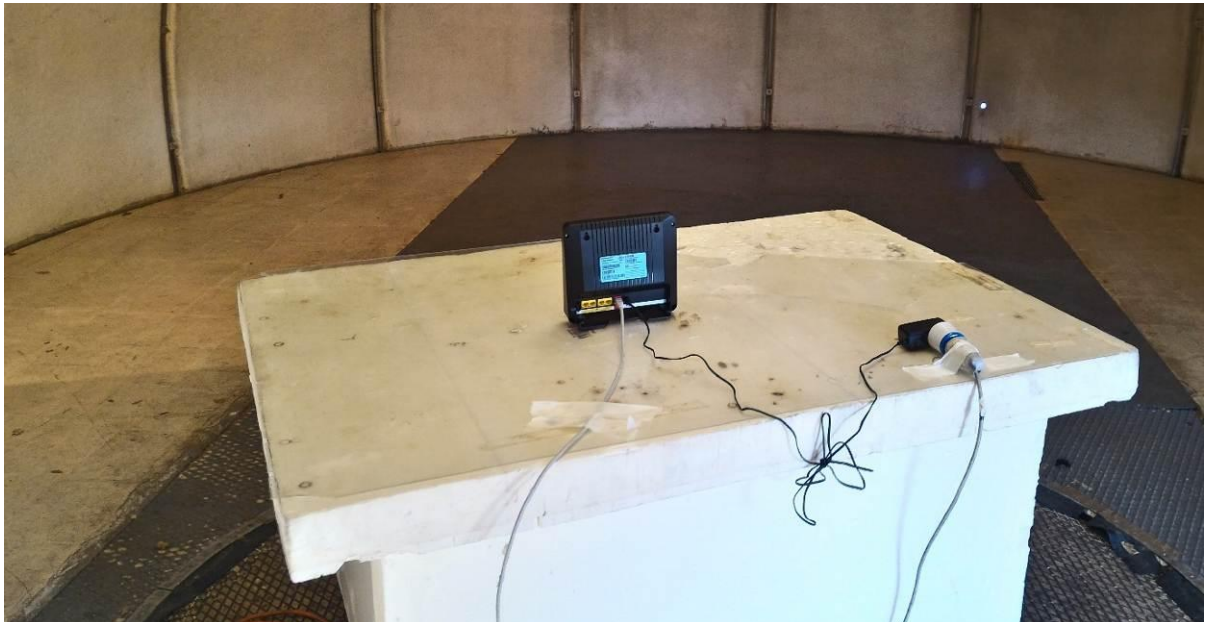
Test setup for radiated field strength ( f < 1\text{GHz} )
