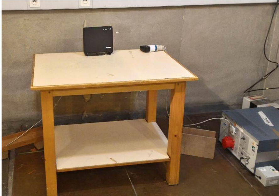
Test setup for power line conducted emissions
