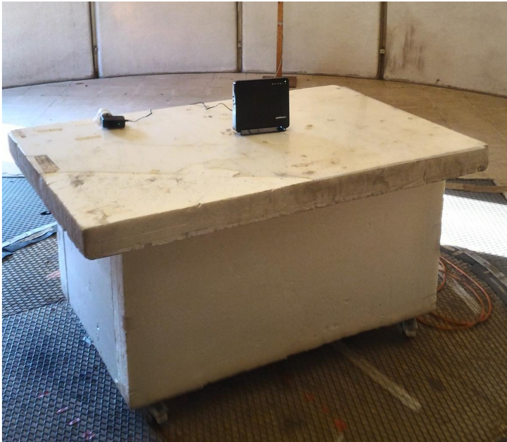
Test setup for radiated field strength ( f < 1\text{GHz} )
