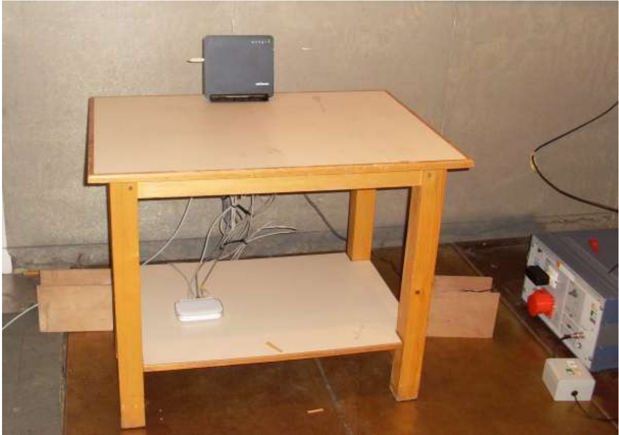
Test setup for power line conducted emissions
