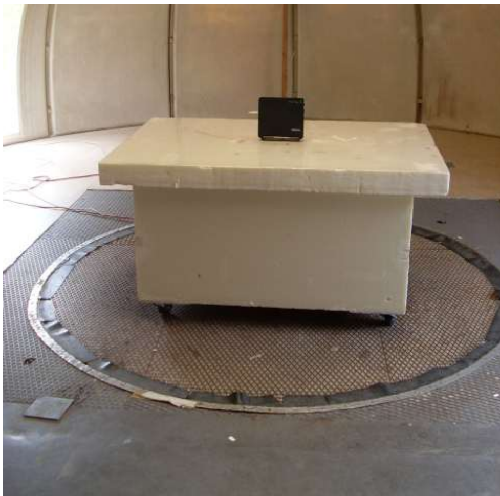
Test setup for radiated field strength
