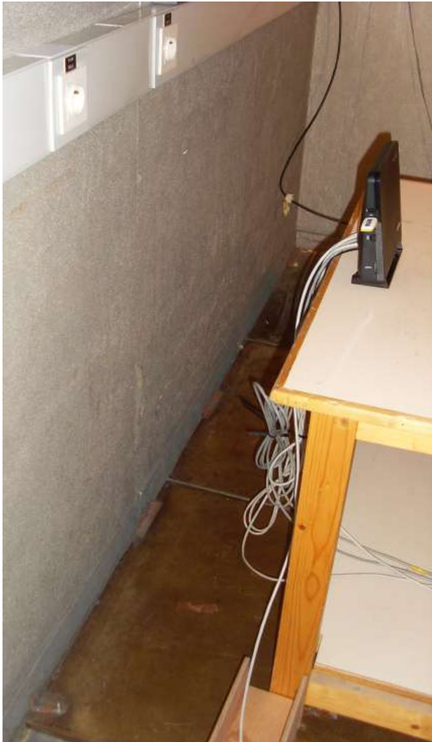
Test setup for power line conducted emissions
