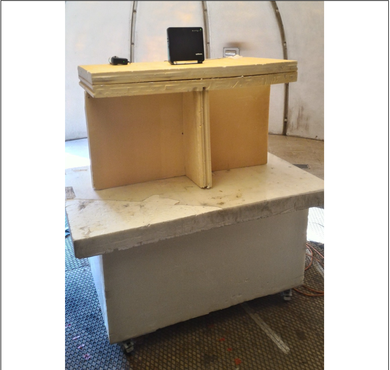
Measurement of radiated disturbances above 1GHz
