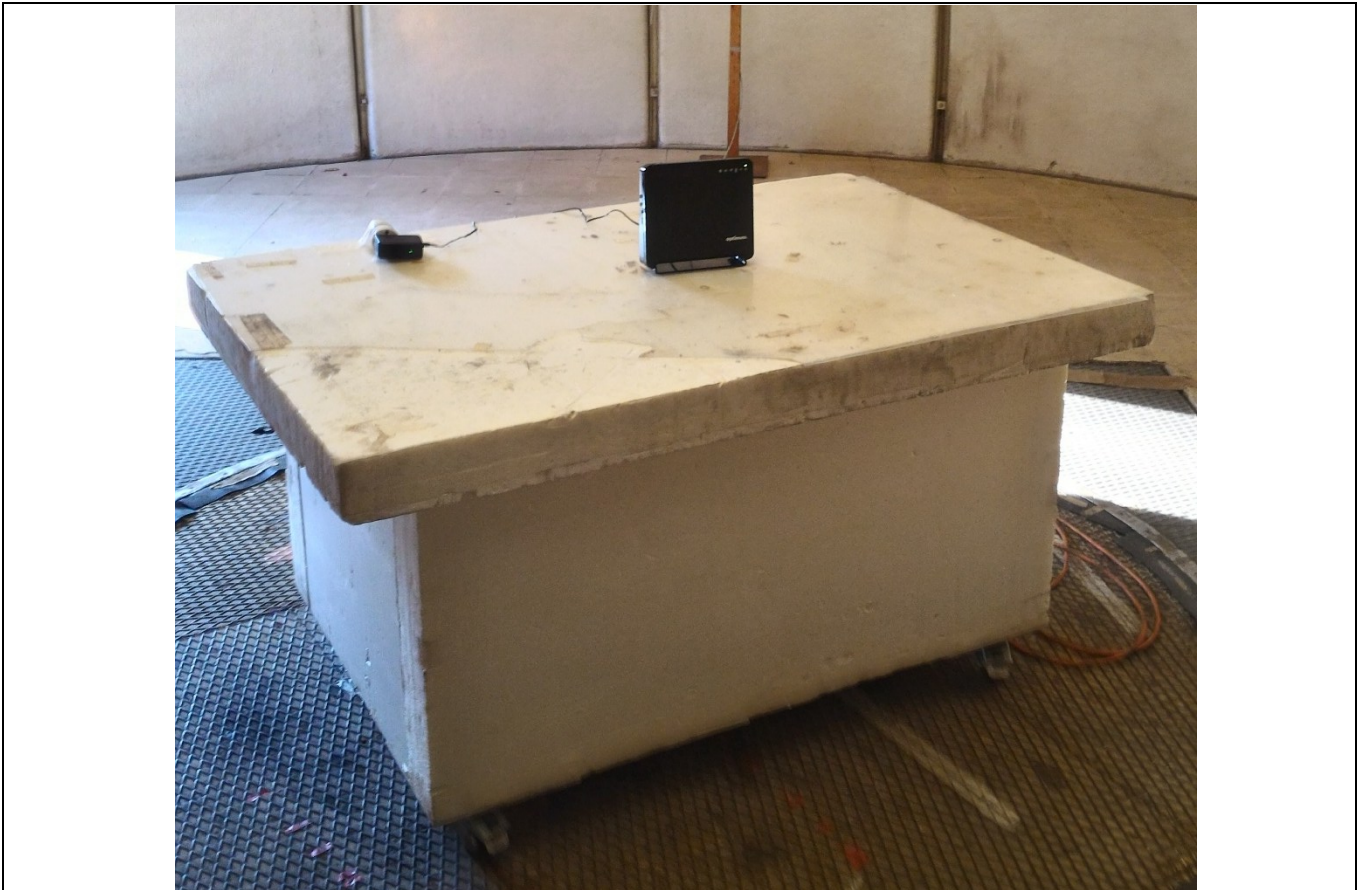
Measurement of radiated disturbances below 1GHz
