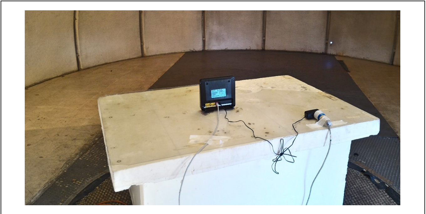
Measurement of radiated disturbances below 1GHz
