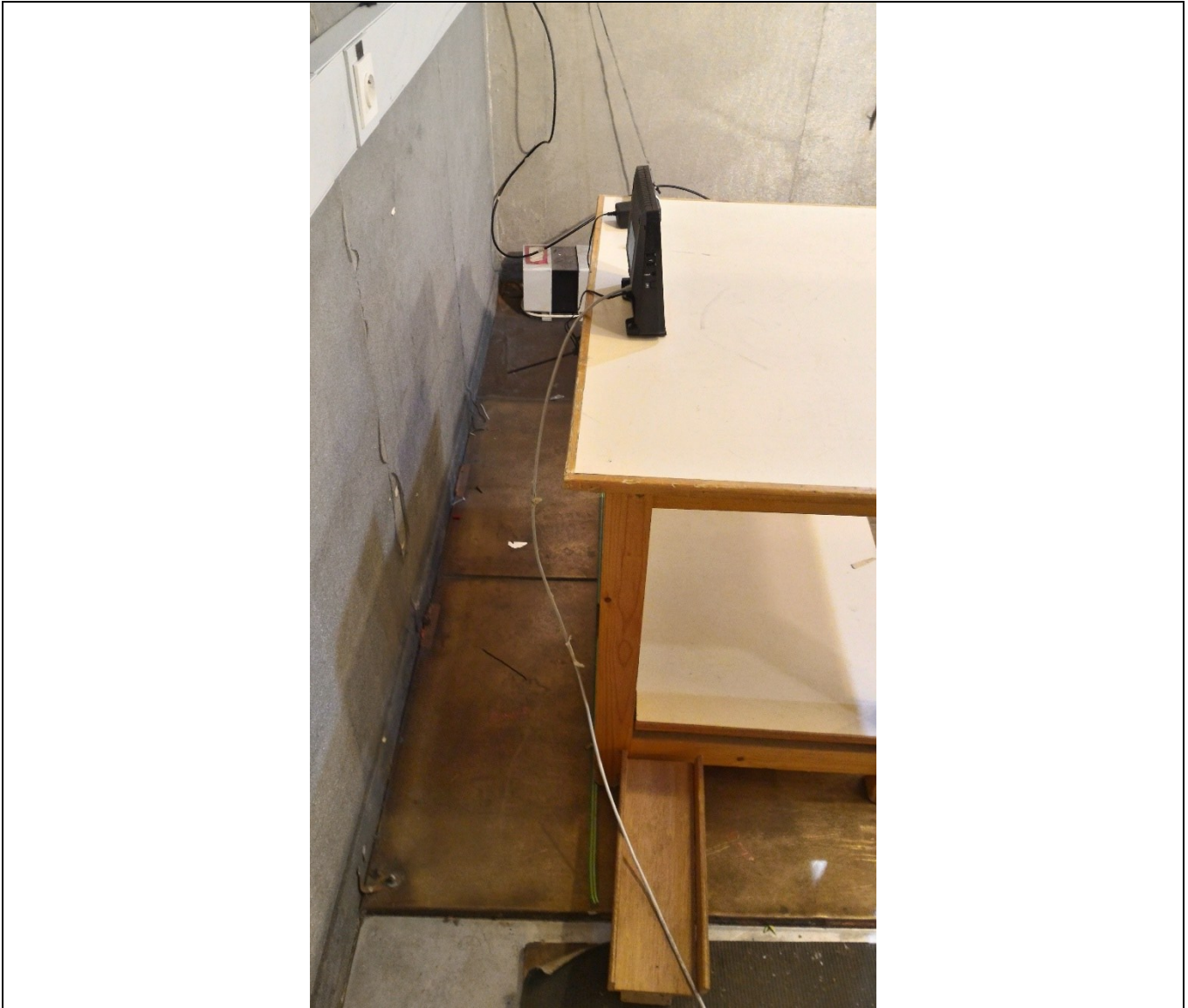
Test set up of conducted emission on power supply
