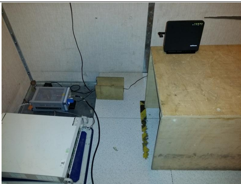
Photograph for AC Power Line Conducted Emissions (Front view)
