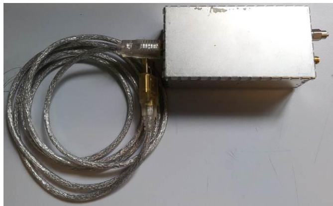
Client Device: CISCO LINKSYS AC530 inside the Shielded Box
