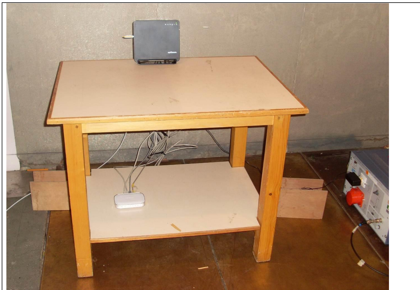
Photograph for AC Power Line Conducted Emissions (Front view)
